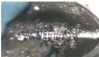
Tungsten Electrodes Eroded
