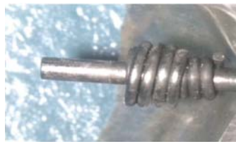
Tungsten Electrodes Intact
